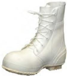
The Extreme Cold Weather boot (ECWB) is constructed with insulation consisting of three layers of needle punched polyester foam hermetically sealed within an outer and inner layer of rubber. The boot is provided with a pressure release valve to adjust internal air pressure in the boot during high altitude operations.
